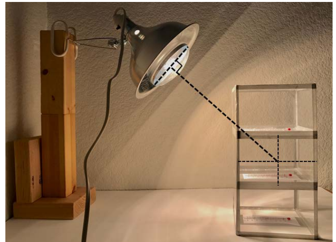
Figure 5. Photograph of control model testing apparatus with indication of light bulb direction
