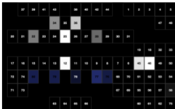
Figure 11, Light board perspective for Cue 36. Light 22, 28, 34, 36 are PAR lights above the stage that represent mock window isolations; Light 25 operates as a ghost light; Lights 45 and 46 are mock side lights. Lights 76 through 80 are LED lights.
