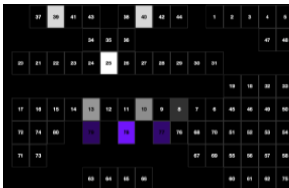
Figure 17 , Light board perspective for Cue 80. Lights 39 and 40 yellow cyc; Light 25 operates as a ghost light; Lights 12, 10, 8 are ERS lights on the cove; Lights 77 through 79 are LED lights.
